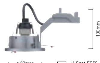
Hi-Spot ES50 Dimensions d'encastrement minimales: 400x400x100mm
